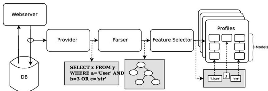
Fig. 5. Overview of the database anomaly detection component.
