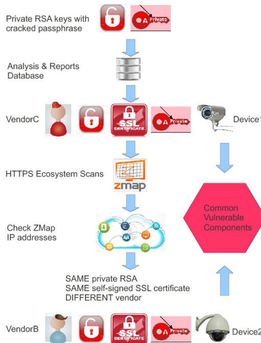
**Figure 4:** Correlation engine and shared self-signed certificates clustering.
